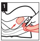
Thread both vehicle lap and shoulder belts through the slot (as shown) and out other side. Buckle. Pull up on shoulder belt until all slack is out and lap belt is tight.
